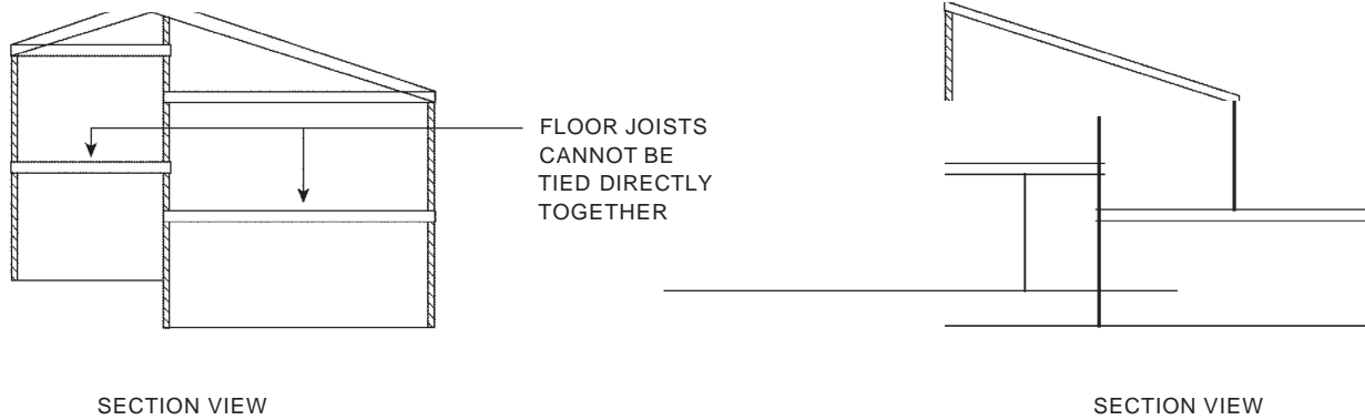
FIGURE 2308.12.6(6) PORTIONS OF FLOOR LEVEL OFFSET VERTICALLY
